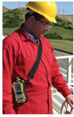
MultiRAE used for worker exposure monitoring at an oil refinery
