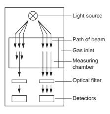
The NDIR sensor element consists of a light source, optical band filters, and detectors. The light source emits a pulsing, wide-band spectrum. The light beams pass through the measuring chamber, and the substance being monitored enters it by diffusion.
